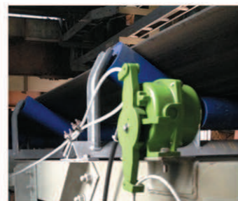
Motor-operated Adjusting Carrier for adjusting belt misalignment
