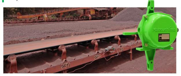
The Pull Cord Switch can stop the belt conveyor at any position because this switch is so made that it is installed at the side of belt conveyor and that the pull cord is mounted along the conveyor.
