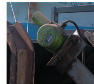
Belt Sway Switch for belt misalignment detection
