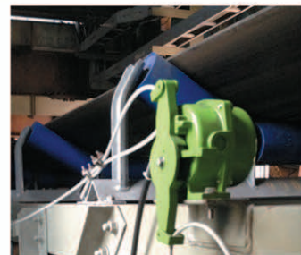
Pull Cord Switch for emergency conveyor stop
