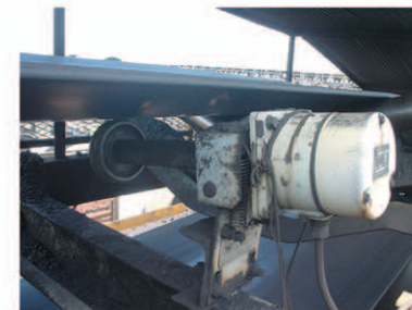
Speed Relay for conveyor slip detection
