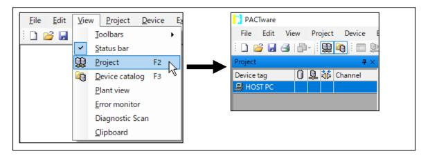
Move the cursor to "HOST PC" in the Project screen, right click and click the item "Add device". The Device for screen will be displayed. Please select "HART Communication" and click the OK button. "COM \*" is displayed under "HOST PC" in the Project screen.
