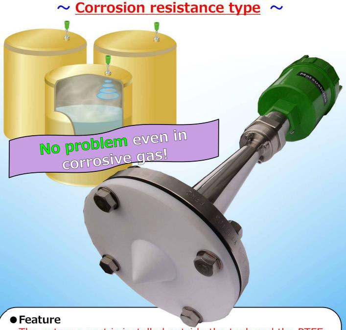
The antenna part is installed outside the tank and the PTFE plate isolates from the process condition. This construction results in stable level measurement without corrosion even in corrosive gas application.
