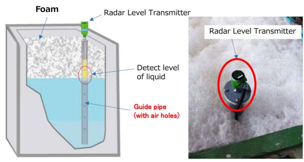
%Drawing and Photo : Detect bubble-free liquid level in the guide pipe
