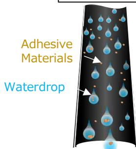
Although it is easy to build up the material in the chute because of high humidity, the special coated antenna prevent the material adhesion inside the antenna.
