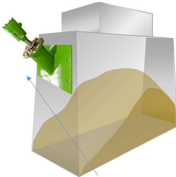
A mounting base fitting with the chute dimension
