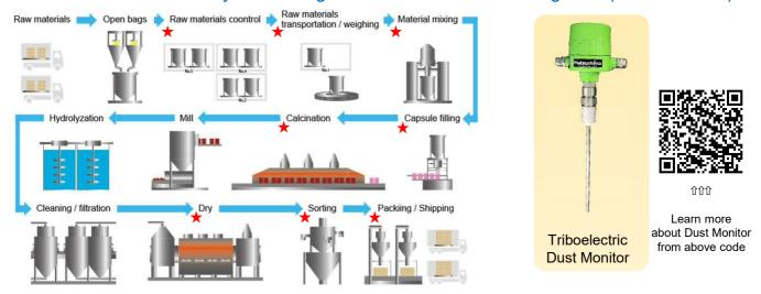
In Lithium-ion battery positive electrode material manufacturing plants, since **Dust Monitor continuously monitors the leakage amount** in dust collectors of the raw material hoppers in each process, the **predictive maintenance** prevents raw material loss to monitor the performance of the bug filter and the wearing tendency of the filter.
